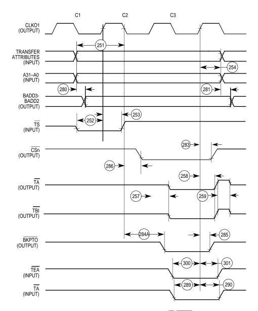
NOTE:  $\underline{\text{MC}68040}$  Transfer Attribute Signals = SIZx, TTx, TMx, R/W,  $\overline{\text{LOCK}}$   $\overline{\text{OE}}$  and  $\overline{\text{WE}}$  are not supported when TSS40 is set to 1
