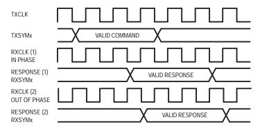
Figure 8-1. Parallel Command Response Time
