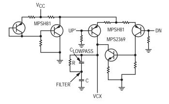
Figure 5-5B. Charge Pump/Filter
