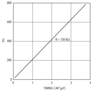
Figure 9–7. Jabber Time Constant versus Capacitance
