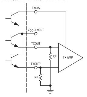
Figure 3-1. Transmitter Outputs
