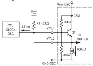
Figure 3–5. TTL Compatible Clock Source Driving CBM
