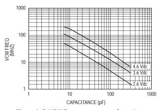
Figure 9-5. VCM Frequency versus Capacitance
