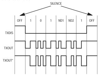
Figure 3-2. Transmitter Output Signaling
