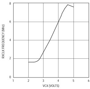
Figure 9–4. VCM Frequency versus Control Voltage (V<sub>CC</sub> = 5.0 Vdc & C = 68 pF)
