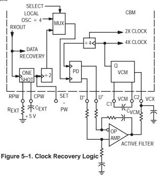
beginning of a transmission can be invalid because the PLL clocks are not sync'ed. As a result the data recovery logic forces silence for 17–18 bit times after the carrier detect switches the reference clock (via the multiplexer) at the beginning of a received transmission.
