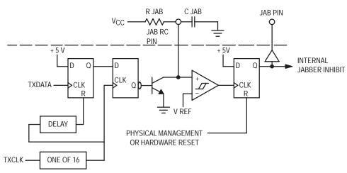
Figure 3-3. Jabber Inhibit Block Diagram
