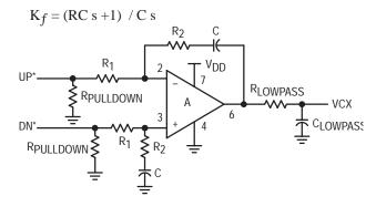
Figure 5-5A. Active Filter Using Op Amp
