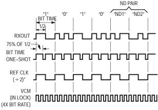
\*NOTE: Ref clock can also be  $180^{\circ}$  out of phase with bit time.
