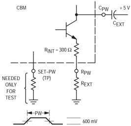
Figure 5-3. One-Shot Timing Components
