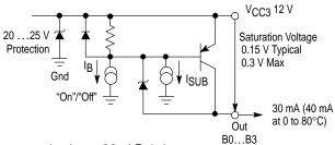
**NOTES:**  $I_B + I_{SUB} = 5.5 \text{ mA Typical}$ I<sub>B</sub> = Base Current
