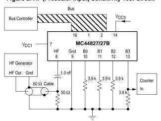
**NOTES**: 1. Device is in test mode. B2, B3 are "On" and B0, B1 are "Off".
