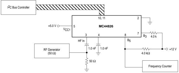
Device is in test mode, B $_5$  and B $_3$  are "On", B $_1$  is "Off". Sensitivity is the level of the HF generator on 50  $\Omega$  load.
