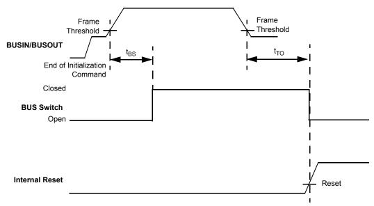
Figure 2. Bus Switch and Reset Timing
