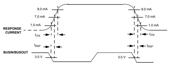
Figure 3. Response Current Timing
