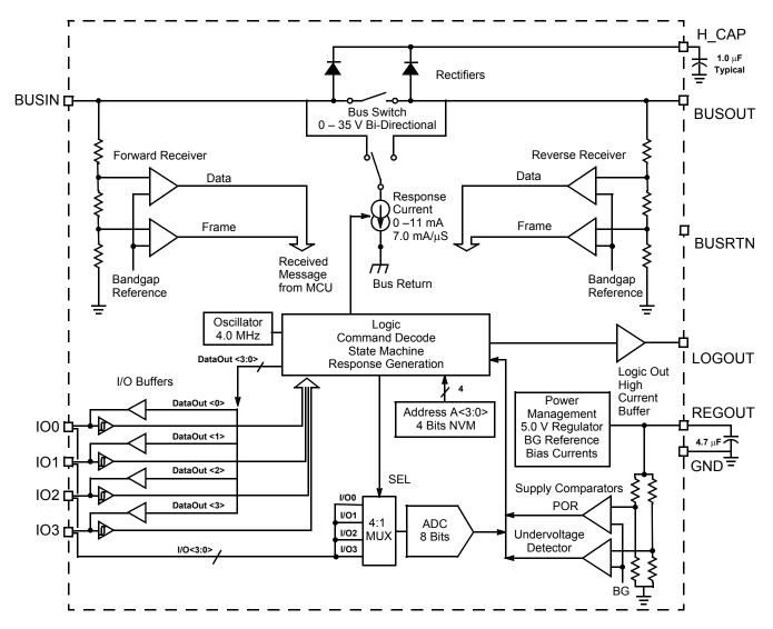
Figure 1. 33793 Simplified Block Diagram
