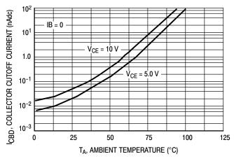
Figure 1. Collector Cutoff Current versus Temperature (Each Transistor)
