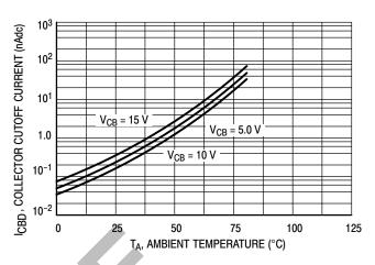
Figure 2. Collector Cutoff Current versus Temperature (Each Transistor)
