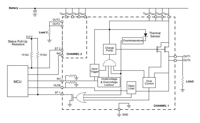
Figure 1. 33289 Simplified Block Diagram
