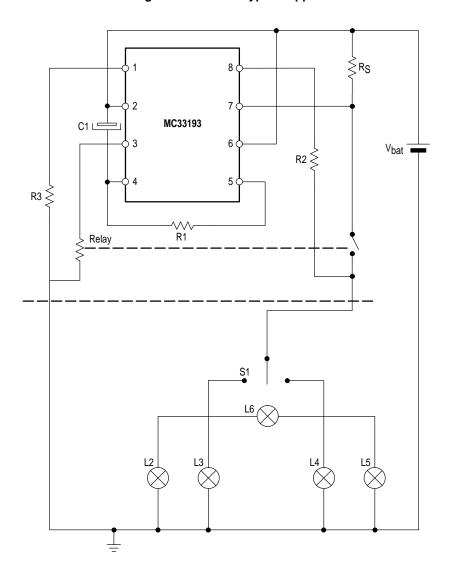
$\begin{aligned} R_S &= 20 \text{ m}\Omega \\ R1 &= 75 \text{ k}\Omega \\ C1 &= 5.6 \text{ }\mu\text{F} \end{aligned}$
