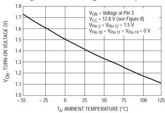
Figure 4. Reference Voltage versus Temperature
