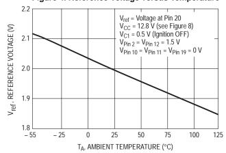
Figure 5. 0TC Reference Voltage versus Temperature
