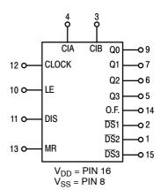
Figure 1. Block Diagram
