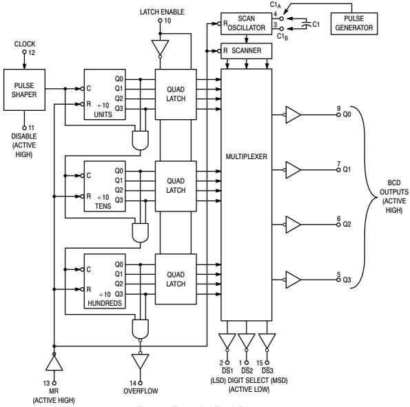
Figure 4. Expanded Block Diagram
