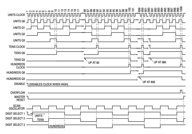
Figure 2. 3-Digit Counter Timing Diagram (Reference Figure 4)
