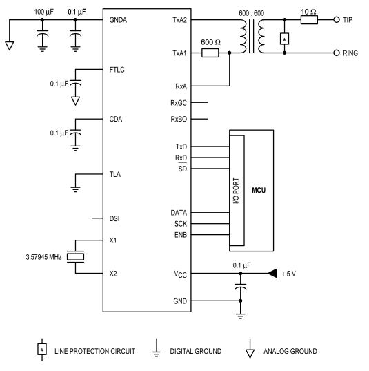
Figure 5. Application Circuit
