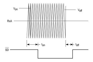
Figure 4. Carrier Detect Timing
