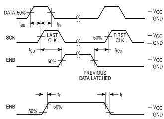
Figure 2. Switching Characteristics
