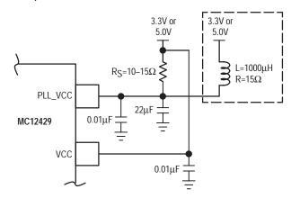
**Figure 6. Power Supply Filter**
