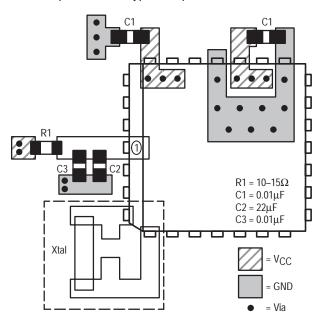
Figure 7. PCB Board Layout for MC12429 (28 PLCC)
