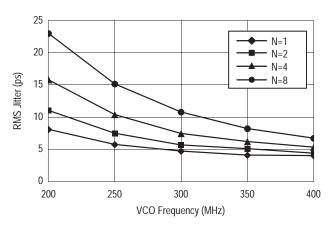
Figure 8. RMS PLL Jitter versus VCO Frequency
