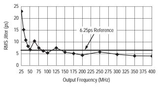
Figure 9. RMS Jitter versus Output Frequency
