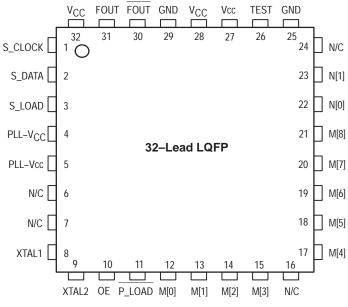
Figure 2. 32–Lead Pinout (Top View)
