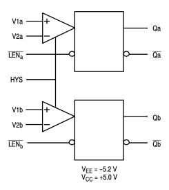
Figure 2. Logic Diagram
