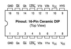
Warning: All  $V_{CC}$ , GND, and  $V_{EE}$  pins must be externally connected to Power Supply to guarantee proper operation.
