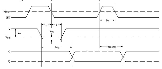
Figure 5. Input/Output Timing Diagram
