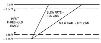
Figure 6. ECL Dispersion Test Input Conditions
