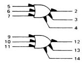
$\begin{array}{l} V_{CC1} = Pin \ 1, \ 15 \\ V_{CC2} = Pin \ 16 \\ V_{EE} = Pin \ 8 \end{array}$
