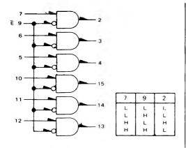
$V_{CC1} = Pin 1 = -1.25 Vdc$  $V_{CC2} = Pin 16 = Gnd$
