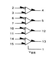
$\begin{array}{rl} {Gnd} &= {Pin} \ 16 \\ {V_{CC}} \ (+5.0 \ Vdc) &= {Pin} \ 9 \\ {V_{EE}} \ (-5.2 \ Vdc) &= {Pin} \ 8 \end{array}$
