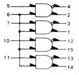
Gnd = Pin 16  $V_{CC} (+5.0 \text{ Vdc}) = Pin 9$  $V_{EE} (-5.2 \text{ Vdc}) = Pin 8$
