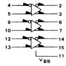
V<sub>CC1</sub> = Pin 1 V<sub>CC2</sub> = Pin 16 V<sub>EE</sub> = Pin 8
