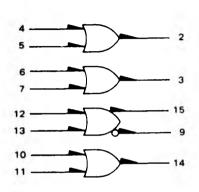
V<sub>CC1</sub> = Pin 1 V<sub>CC2</sub> = Pin 16 V<sub>EE</sub> = Pin 8
