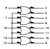
$\begin{array}{l} V_{CC1} = Pin \quad 1 \\ V_{CC2} = Pin \quad 16 \\ V_{EE} = Pin \quad 8 \end{array}$
