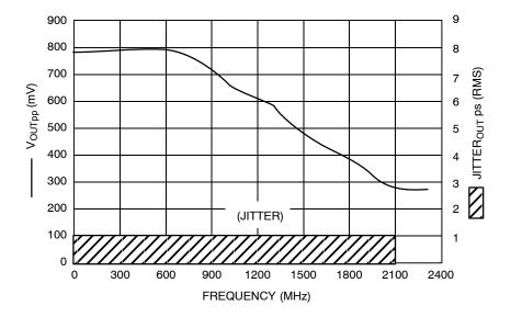
Figure 3. F<sub>max</sub>/Jitter
