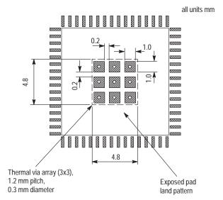
Figure 7. Recommended solder mask openings
