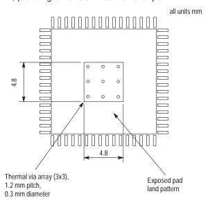
Figure 6. Recommended thermal land pattern
