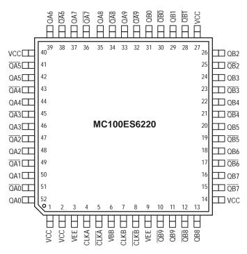
Figure 1. MC100ES6220 Logic Diagram
