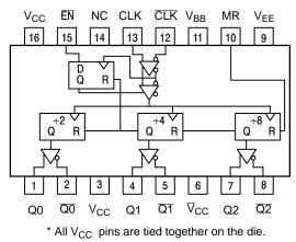
Warning: All  $V_{CC}$  and  $V_{EE}$  pins must be externally connected to Power Supply to guarantee proper operation.
