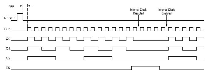
The EN signal will freeze the internal clocks to the flip–flops on the first falling edge of CLK after its assertion. The internal dividers will maintain their state during the internal clock freeze and will return to clocking once the internal clocks are unfrozen. The outputs will transition to their next states in the same manner, time and relationship as they would have had the EN signal not been asserted.
