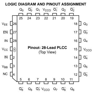
$^{\ast}$  All V\_CC and V\_CCO pins are tied together on the die.
