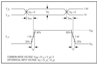
Figure 3. Propagation Delay and Transition-Time Waveforms
