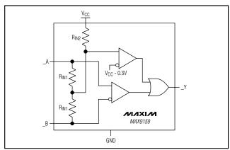
Figure 1. Input Fail-Safe Network
