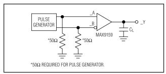
Figure 2. Propagation Delay and Transition-Time Test Circuit
