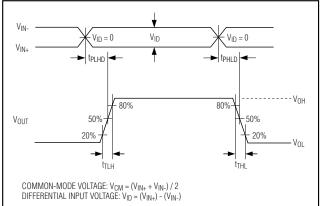
Figure 3. Propagation Delay and Transition-Time Waveforms
