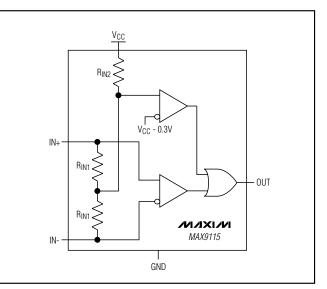
Figure 1. Input Fail-Safe Network
