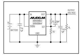
Figure 2. Adjustable Output Using External Feedback Resistors
