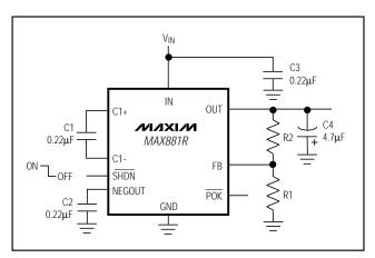
Figure 4. Adjustable Output Configuration
