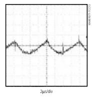
$V_{IN}$  = 3.3V,  $V_{OUT}$  = -3.18V,  $I_{OUT}$  = 5mA, 20mV/div, AC COUPLED
