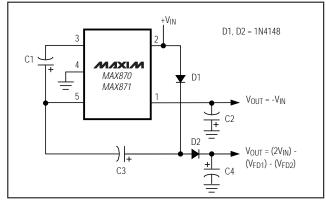
Figure 6. Combined Doubler and Inverter
