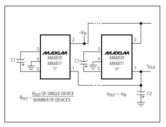
Figure 5. Paralleling MAX870s or MAX871s to Reduce Output Resistance
