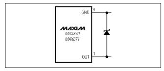
Figure 7. High V- Load Current
