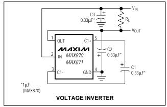
Figure 1. Test Circuit
