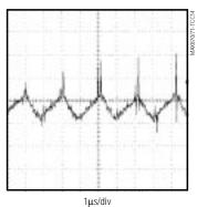
$V_{IN} = 3.3V$ ,  $V_{OUT} = -3.14V$ ,  $I_{OUT} = 5mA$ , 20mV/div, AC COUPLED
