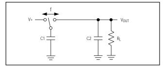
Figure 3a. Switched-Capacitor Model
