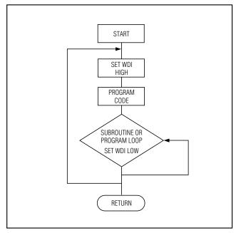
Figure 5. Watchdog Flow Diagram
