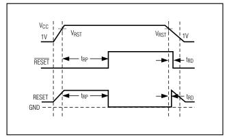
Figure 2. Reset Timing Diagram
