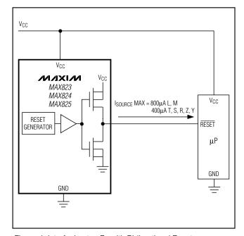
Figure 4. Interfacing to μPs with Bidirectional Resets
