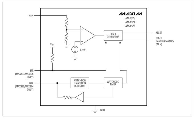
Figure 1. Functional Diagram
