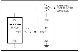
Figure 3. Interfacing to µPs with Bidirectional Reset I/O
