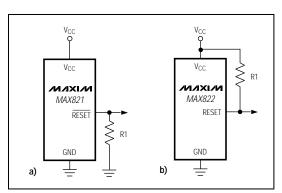
Figure 2. RESET/RESET Valid to V<sub>CC</sub> = Ground Circuit
