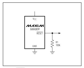
Figure 2.  $\overline{RESET}$  Valid to  $V_{CC}$  = Ground Circuit
