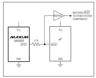
Figure 3. Interfacing to μPs with Bidirectional Reset I/O
