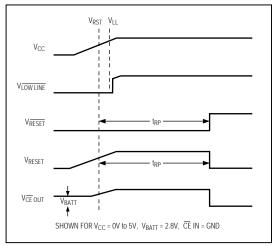
Figure 2a. Timing Diagram, V<sub>CC</sub> Rising
