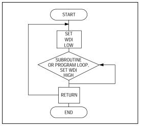
Figure 16. Watchdog Flow Diagram
