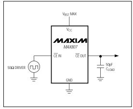
Figure 8. CE Propagation Delay Test Circuit
