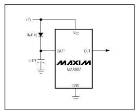
Figure 13. SuperCap or MaxCap on BATT
