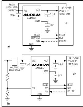
Figure 11. a) If the preregulated supply is inaccessible,  $\overline{\text{LOW}}$  LINE generates the NMI for the  $\mu\text{P}$ . b) Use  $\overline{\text{PFO}}$  to generate the  $\mu\text{P}$  NMI if the preregulated supply is accessible.
