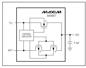
Figure 12. V<sub>CC</sub> and BATT-to-OUT Switch
