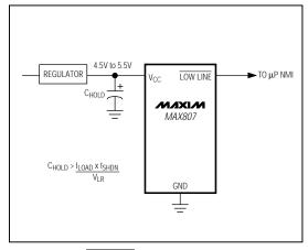
Figure 9. Using  $\overline{\text{LOW LINE}}$  to Provide a Power-Fail Warning to the  $\mu\text{P}$
