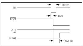
Figure 4. Manual-Reset Timing Diagram
