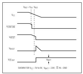
Figure 2b. Timing Diagram, VCC Falling
