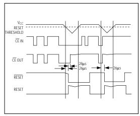
Figure 7. Reset and Chip-Enable Timing
