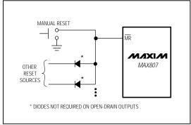
Figure 3. Diode "OR" connections allow multiple reset sources to connect to  $\overline{\textit{MR}}.$
