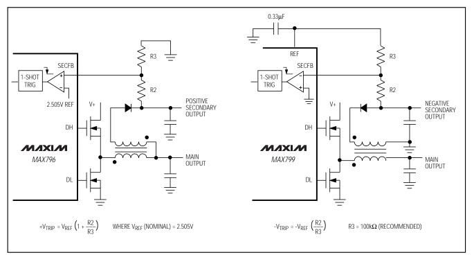
Figure 9. Secondary-Output Feedback Dividers, MAX796 vs. MAX799
