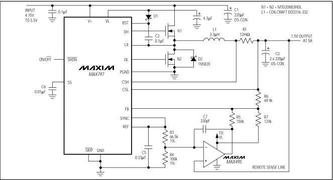
Figure 21. 1.5V GTL Bus Termination Supply
