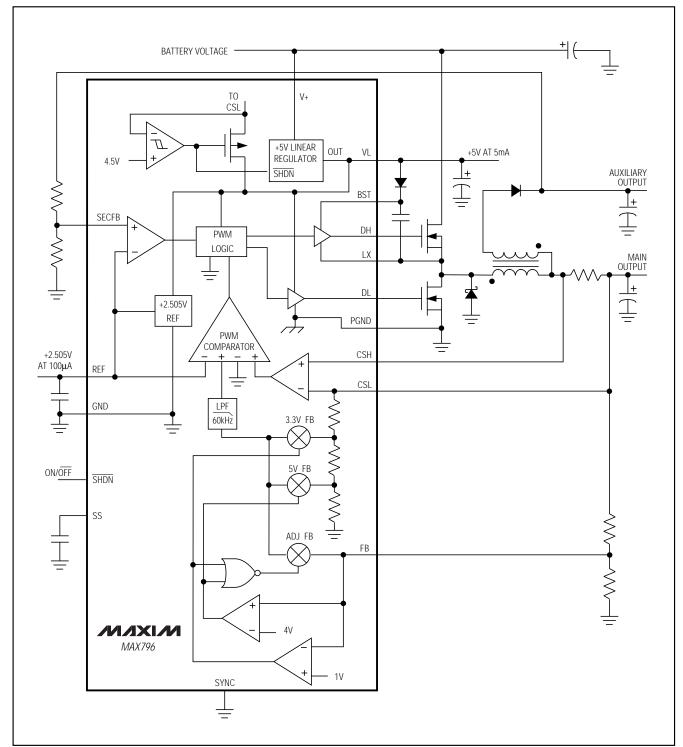
Figure 2. MAX796 Block Diagram
