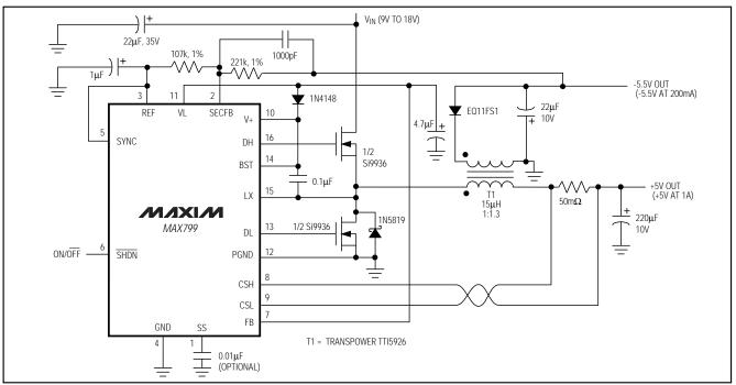
Figure 13. ±5V Dual-Output Application (MAX799)
