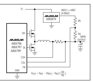
Figure 7. Output Voltage Less than 2.5V
