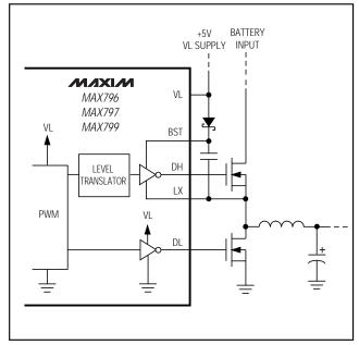
Figure 5. Boost Supply for Gate Drivers
