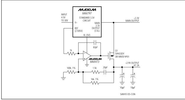
Figure 14. 2.9V Low-Dropout Linear Regulator with Fast Transient Response
