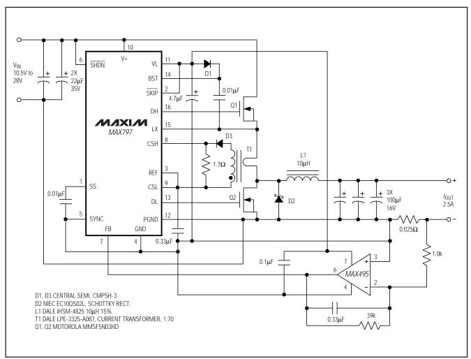
Figure 22. Battery-Charger Current Source
