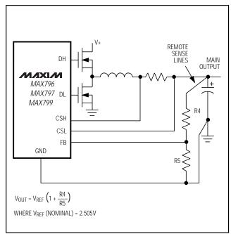
Figure 6. Adjusting the Main Output Voltage
