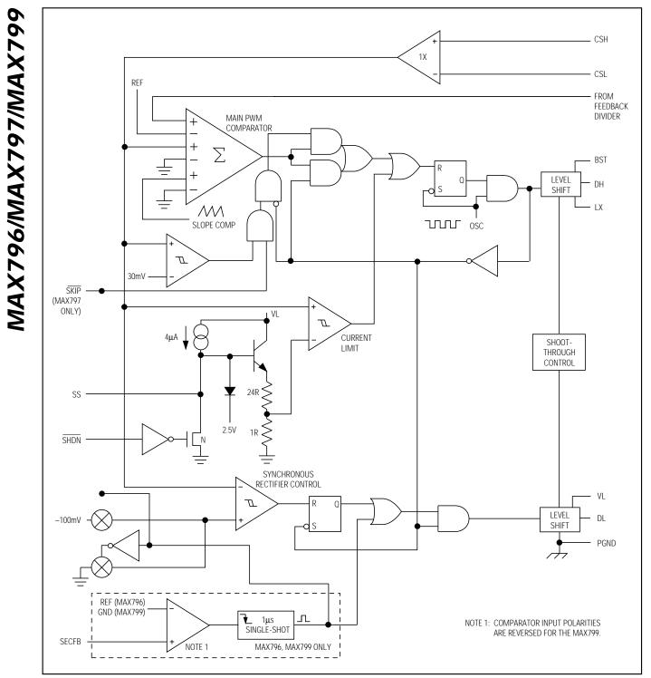
Figure 3. PWM Controller Detailed Block Diagram
