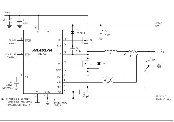
Figure 1. Standard 3.3V Application Circuit
