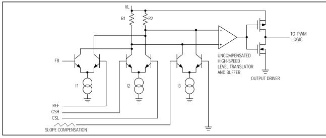
Figure 4. Main PWM Comparator Block Diagram
