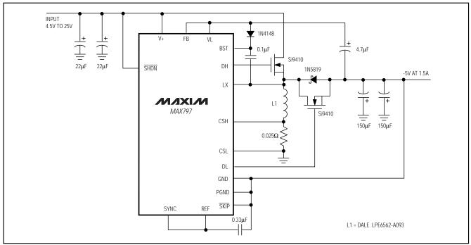
Figure 19. Negative-Output (Inverting Topology) Power Supply
