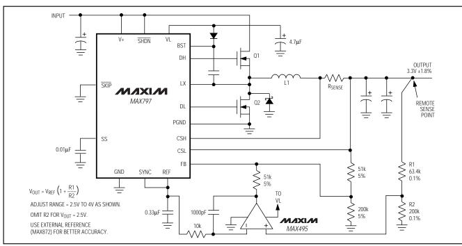
Figure 18. High-Accuracy Adjustable-Output Application
