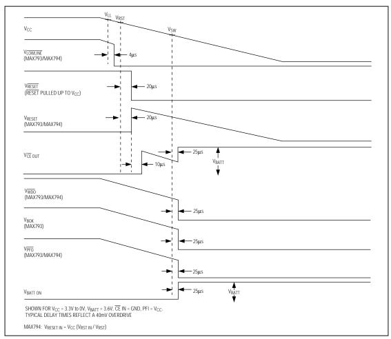
Figure 2. Timing Diagram, VCC Falling
