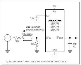
Figure 9. CE Propagation Delay Test Circuit
