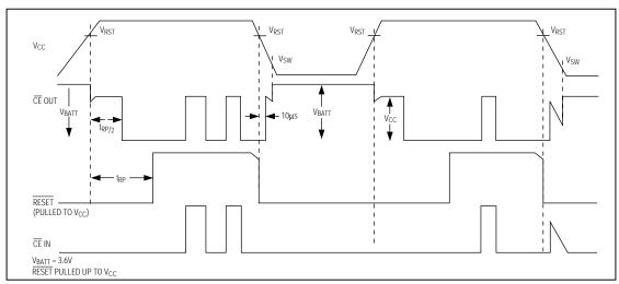
Figure 8. Chip-Enable Timing
