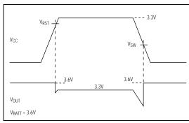
Figure 13. Battery Switchover Timing
