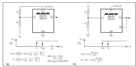
Figure 12. Using the Power-Fail Comparator to Monitor an Additional Power Supply: (a) V<sub>IN</sub> Is Negative, (b) V<sub>IN</sub> Is Positive
