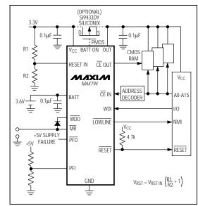
Figure 3. MAX794 Standard Application Circuit
