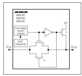
Figure 7. Chip-Enable Transmission Gate
