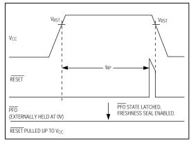
Figure 4. Battery Freshness Seal Enable Timing
