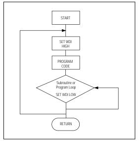
Figure 19. Watchdog Flow Diagram
