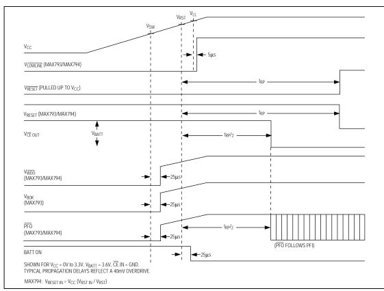
Figure 1. Timing Diagram, V<sub>CC</sub> Rising
