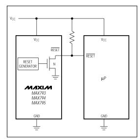
Figure 17. Interfacing to μPs with Bidirectional Reset I/O
