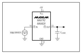
Figure 10. CE Propagation Delay Test Circuit
