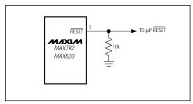
Figure 5. Adding an external pull-down resistor ensures  $\overline{\textit{RESET}}$  is valid with  $V_{CC}$  down to GND.
