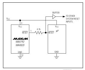
Figure 12. Interfacing to μPs with Bidirectional **RESET** Pins
