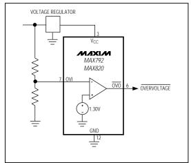
Figure 6. Detecting an Overvoltage Condition
