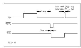
Figure 7. WDI, WDO and WDPO Timing Diagram
