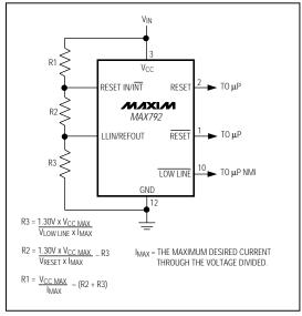
Figure 4b. Connection for External Threshold Programming Mode
