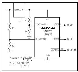
Figure 4c. Alternative connection for external programming mode
