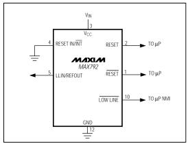
Figure 4a. Connection for Internal Threshold Mode
