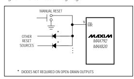
Figure 3. Diode "OR" connections allow multiple reset sources to connect to  $\overline{\textit{MR}}.$
