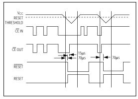
Figure 9. Reset and Chip-Enable Timing
