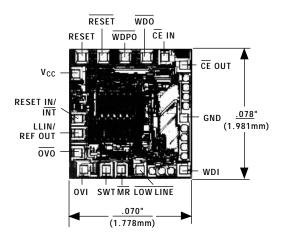
TRANSISTOR COUNT: 950; SUBSTRATE CONNECTED TO V<sub>CC</sub>.
