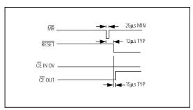
Figure 2. Manual-Reset Timing Diagram
