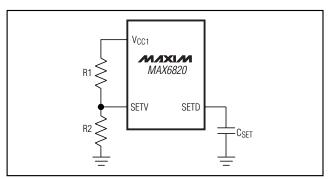
Figure 2. tDFLAY (MAX6820 ONLY) and VTH Adjust
