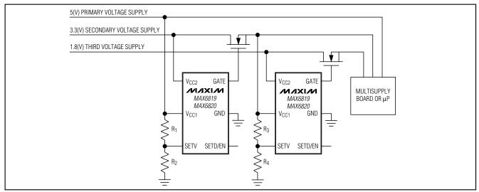
Figure 4. Sequencing Three Power Supplies
