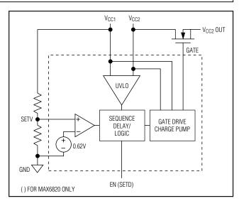
Figure 1. Functional Diagram
