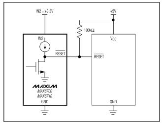
Figure 4. Interfacing to Different Logic-Supply Voltage
