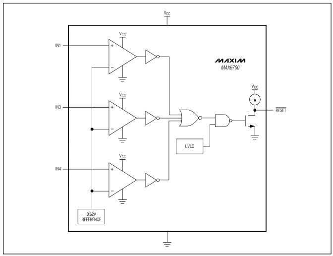
Figure 1. MAX6700 Functional Diagram
