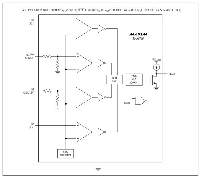
Figure 2. MAX6710 Functional Diagram
