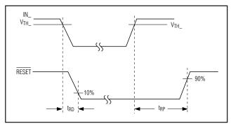
Figure 3. RESET Output Timing Diagram
