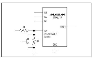
Figure 6. Adding Manual Reset Capability
