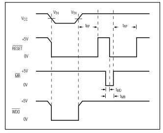
Figure 6. MAX6701(A)/MAX6702(A)/MAX6703(A)/MAX6705(A)/ MAX6706(A)/MAX6707(A) RESET, MR, and WDO Timing with WDI Three-Stated
