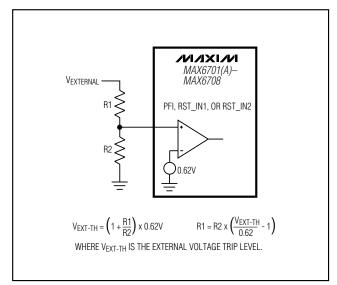
Figure 8. Calculating Adjustable Voltage Thresholds
