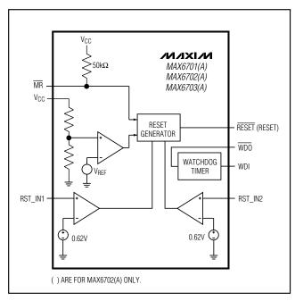
Figure 3. MAX6701(A)/MAX6702(A)/MAX6703(A) Functional Diagram
