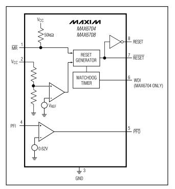
Figure 2. MAX6704/MAX6708 Functional Diagram
