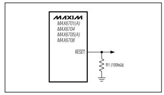
Figure 9. RESET Valid to Ground Circuit
