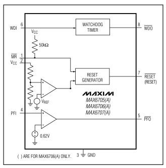
Figure 1. MAX6705(A)/MAX6706(A)/MAX6707(A) Functional Diagram
