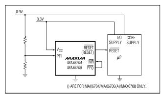
Figure 10. Monitoring Other System Voltages
