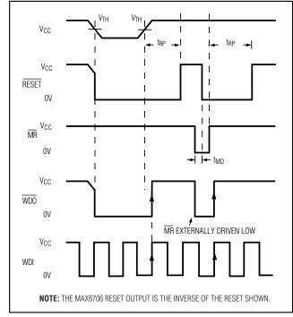
Figure 4. MAX6705/MAX6706/MAX6707 RESET, MR, WDO, and WDI Timing
