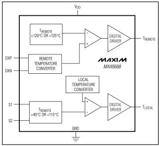
Figure 1b. MAX6688 Functional Block Diagram
