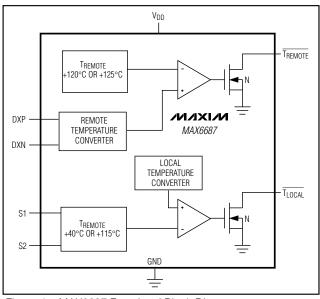
Figure 1a. MAX6687 Functional Block Diagram
