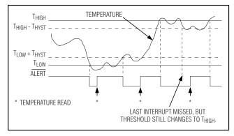
Figure 2. Example of ALERT Operation in Interrupt Mode
