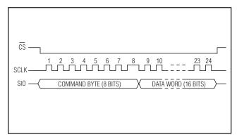
Figure 3. MAX6662 Serial Interface Operation
