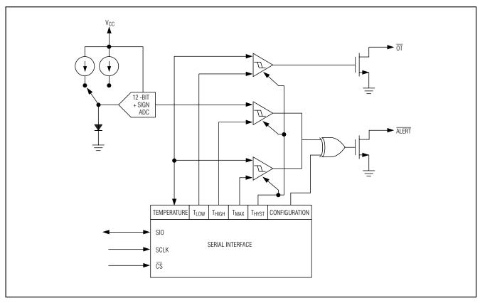
Figure 1. MAX6662 Simplified Functional Diagram
