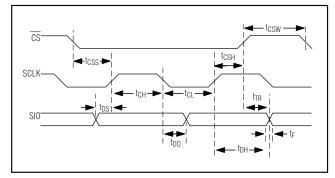
Figure 4. Detailed Serial Interface Timing Diagram
