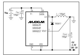
Figure 6. Inverting Configuration
