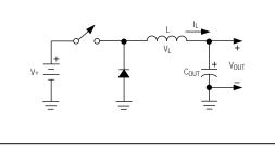
Figure 1. Simplified Step-Down Converter
