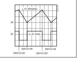
Figure 2. Simplified Step-Down Converter Operation
