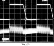
A: V<sub>IN</sub>, 6V TO 11.5V, 2V/div B: V<sub>OUT</sub>, 100mV/div V<sub>OUT</sub> = 5V, I<sub>LOAD</sub> = 100mA
