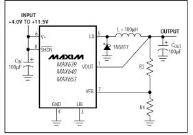
Figure 4. Adjustable-Output Operation
