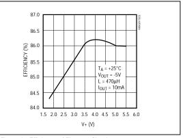
Figure 8. Efficiency of Figure 6 Circuit
