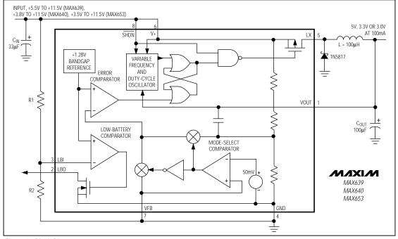
Figure 3. Block Diagram
