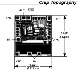
TRANSISTOR COUNT: 221 SUBSTRATE CONNECTED TO V+
