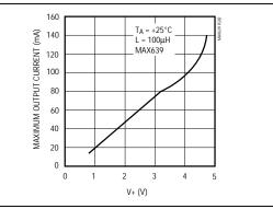
Figure 7. Maximum Current Capability of Figure 6 Circuit
