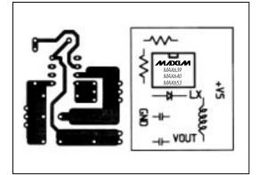
Figure 5. Through-Hole PC Layout and Component Placement Diagram for Standard Step-Down Application (Top-Side View)
