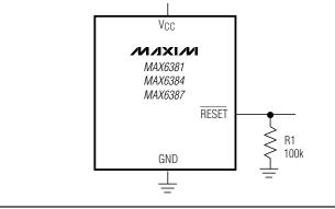
Figure 2. RESET Valid to V<sub>CC</sub> = Ground Circuit
