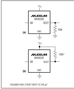
Figure 2. Ensuring Reset Valid down to  $V_{CC} = 0$
