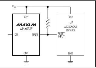
Figure 1. Interfacing to µPs with Bidirectional Reset Pins
