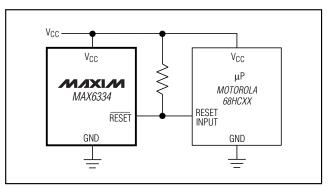
Figure 1. Interfacing to µPs with Bidirectional Reset Pins
