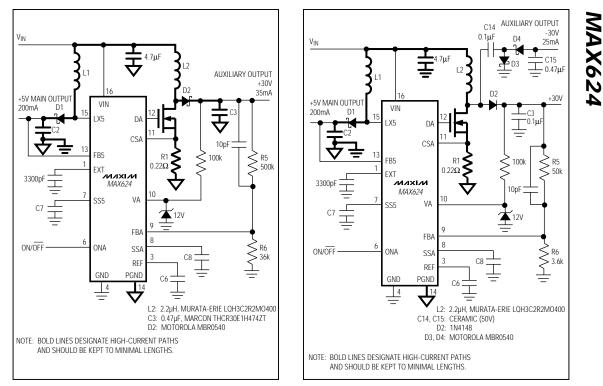
Figure 10. Positive 30V (35mA) Auxiliary Output Application Circuit
