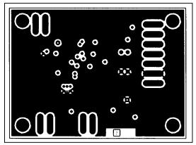
Figure 6. MAX624 PC Board Layout-VSWITCHED Plane
