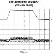
$$\begin{split} &I_{LOAD} = 40\text{mA} \\ &A: \ V_{IN} = 3.3 V \text{ to } 5 V \\ &B: \ 5 V \text{ MAIN OUTPUT (50mV/div, AC-COUPLED)} \end{split}$$
