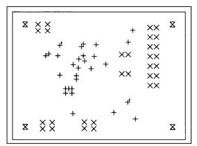
Figure 4. MAX624 PC Board Drill and Mechanical Guide
