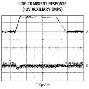
$$\begin{split} &I_{LOAD} = 20 \text{mA} \\ &A: \ V_{IN} = 3.3 \text{V to 5V} \\ &B: \ 12 \text{V} \text{AUXILIARY OUTPUT (200 \text{mV/div}, \text{AC-COUPLED})} \end{split}$$
