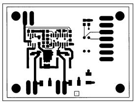
Figure 5. MAX624 PC Board Layout—Component Side
