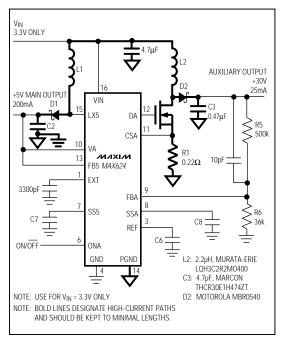
Figure 9. Positive 30V (25mA) Auxiliary Output Application Circuit
