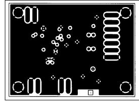
Figure 7. MAX624 PC Board Layout—Ground Plane
