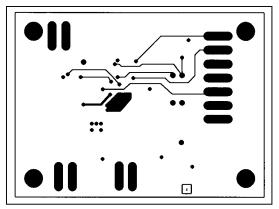
Figure 8. MAX624 PC Board Layout—Solder Side
