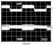
A: I<sub>LOAD</sub> = 0mA to 80mA B: 12V AUXILIARY SMPS (200mV/div, AC-COUPLED)
