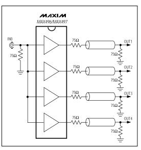
Figure 3. One-to-Four Distribution Amplifier
