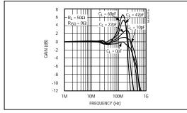
Figure 5a. MAX496 Small-Signal Gain vs. Frequency and Load Capacitor ( $R_L$  = 50 $\Omega$ ,  $R_{ISO}$  = 0 $\Omega$ )
