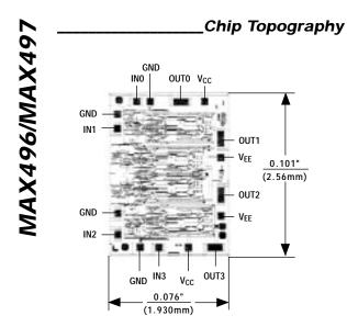
TRANSISTOR COUNT: 544 SUBSTRATE CONNECTED TO VEE
