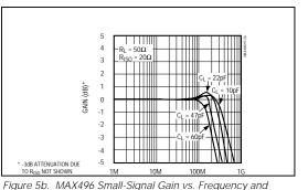
Figure 5b. MAX496 Small-Signal Gain vs. Frequency and Load Capacitor ( $R_L = 50\Omega$ ,  $R_{ISO} = 20\Omega$ )
