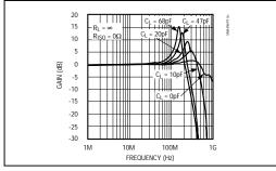
Figure 5c. MAX496 Small-Signal Gain vs. Frequency and Load Capacitor ( $R_L = \infty$ ,  $R_{ISO} = 0\Omega$ )
