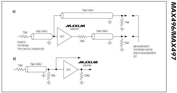
Figure 2. Differential Phase and Gain Error Test Circuits: a) MAX497, Gain of +2 Amplifier; b) MAX496 Unity-Gain Amplifier
