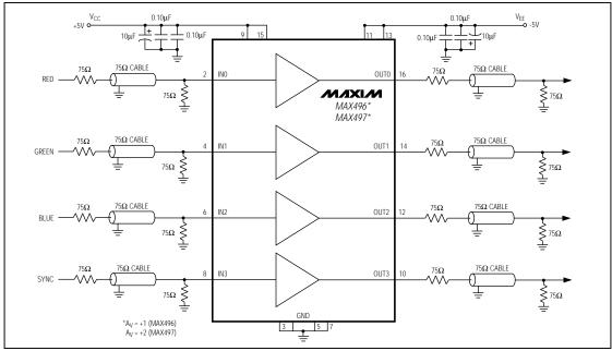
Figure 1. Typical Operating Circuit
