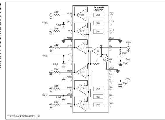
Figure 1. MAX4135 Typical Operating Circuit
