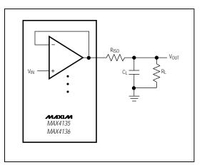
Figure 4. Capacitive-Load Driving Circuit
