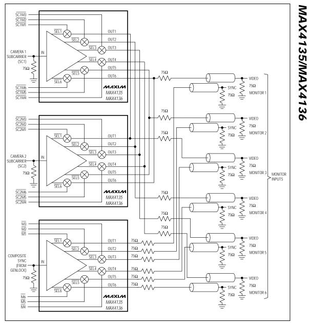
Figure 6. Two Cameras to Six Monitors Distribution Amplifier
