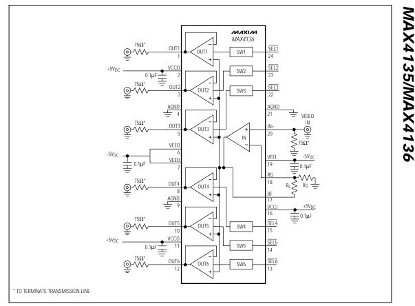
Figure 2. MAX4136 Typical Operating Circuit
