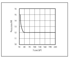
Figure 5. Optimal Isolation Resistor (RISO) vs. CLOAD
