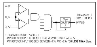
Figure 2b. MAX322\_E with Transmitters Enabled Using AutoShutdown
