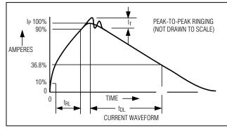
Figure 5b. Human Body Model Current Waveform
