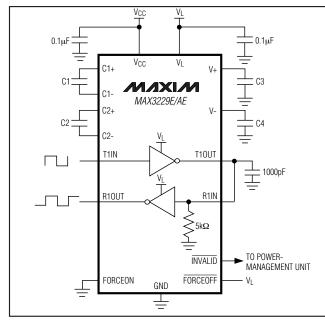
Figure 8. Transmitter Loopback Test Circuit
