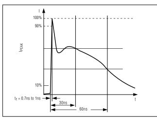
Figure 6b. IEC 1000-4-2 ESD Generator Current Waveform
