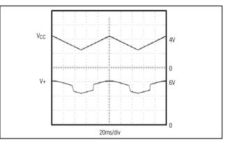
Figure 1. V+ Switchover for Changing V<sub>CC</sub>
