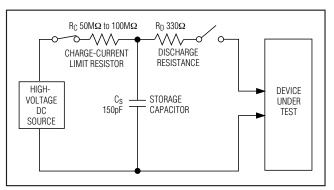
Figure 6a. IEC 1000-4-2 ESD Test Model
