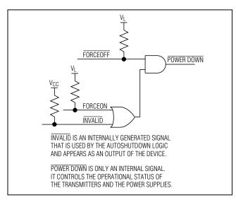
Figure 2c. MAX322\_E AutoShutdown Logic
