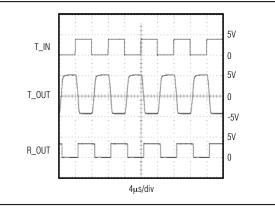
Figure 10. Loopback Test Result at 250kbps
