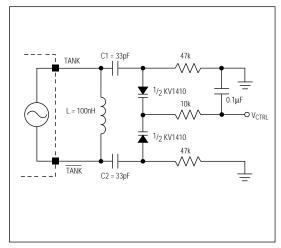
Figure 4. Typical Resonant Tank Circuit
